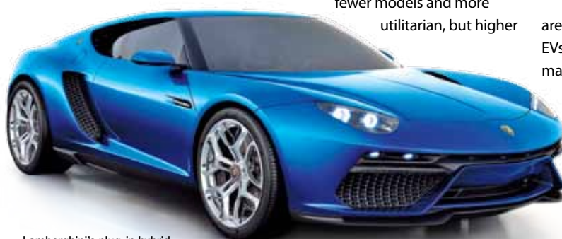
Lamborghini's plug-in hybrid concept, the Asterion LPI 910-4, has a 5.2-litre V10 engine and three electric motors. Thanks to an electric-only range of 50km, it produces emissions of 98g/km. Visit www.autofile.co.nz for more from Paris Motor Show
